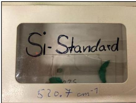
**Figure 12.** Calibration standard silicon.
