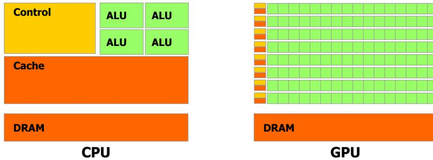
Figure 4.2: Design difference between GPUs and CPUs, taken from [NVI10]
