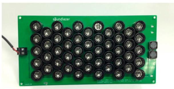
Fig. 5. Transducer's honeycomb array in a Soundlazer's mini parametric speaker board.
