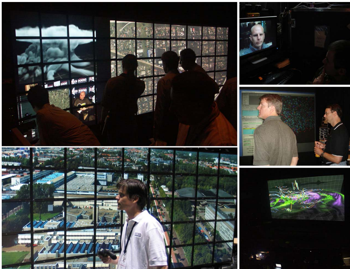
Fig. 1. Top left: SAGE showing several high resolution streams (high-definition thunderstorm simulation; high-definition live video; ultra-high-resolution aerial photography of New Orleans after Hurricane Katrina) simultaneously on the Lambda Vision display; Bottom left: TOPS showing a single high resolution montage of Amsterdam; top right: auto-stereoscopic video conferencing on the Varrier display; middle right: Solutions Server streaming graphics to a passive stereo XGA resolution display; bottom right: BPlayer streaming high-definition stereo movies to a high-definition passive stereo display.
