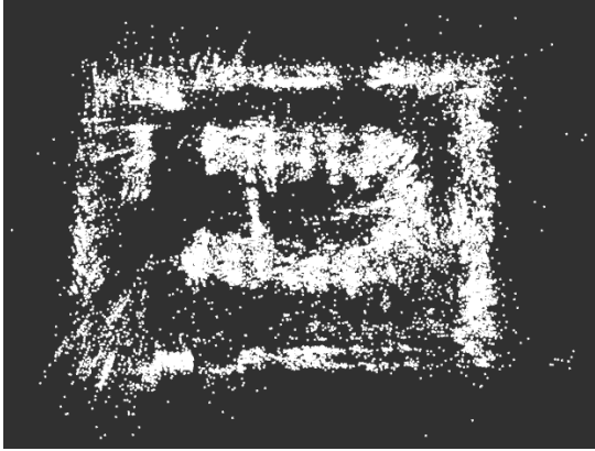
Fig. 6: View from above of the point cloud resulting from the mapping of the laboratory using ORB-SLAM2.
