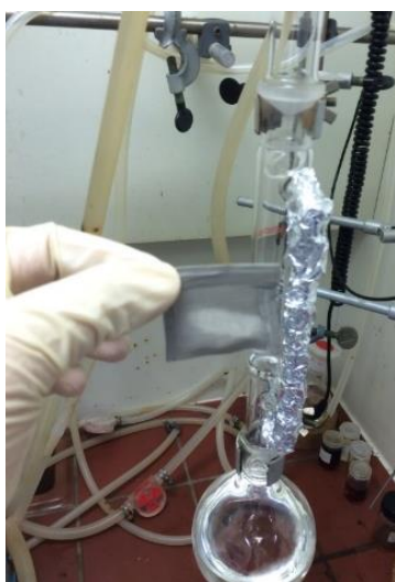
Figure A- 5.4 Assembly of Soxhlet extraction technique and sample preparation (left), and number of cycles used for each blend (right).
