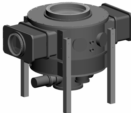
Figure 14. EMIR test cryostat. General view
