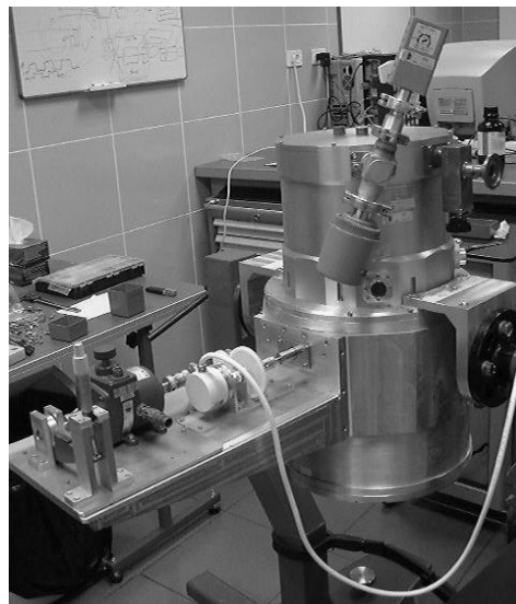
Figure 11. Cryo motors test bench
