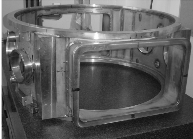
Figure 15. EMCTS main body under manufacturing
