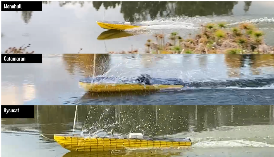
Figure 5.24: Lateral photograph of the three models at cruising speed (5.3 m/s).
