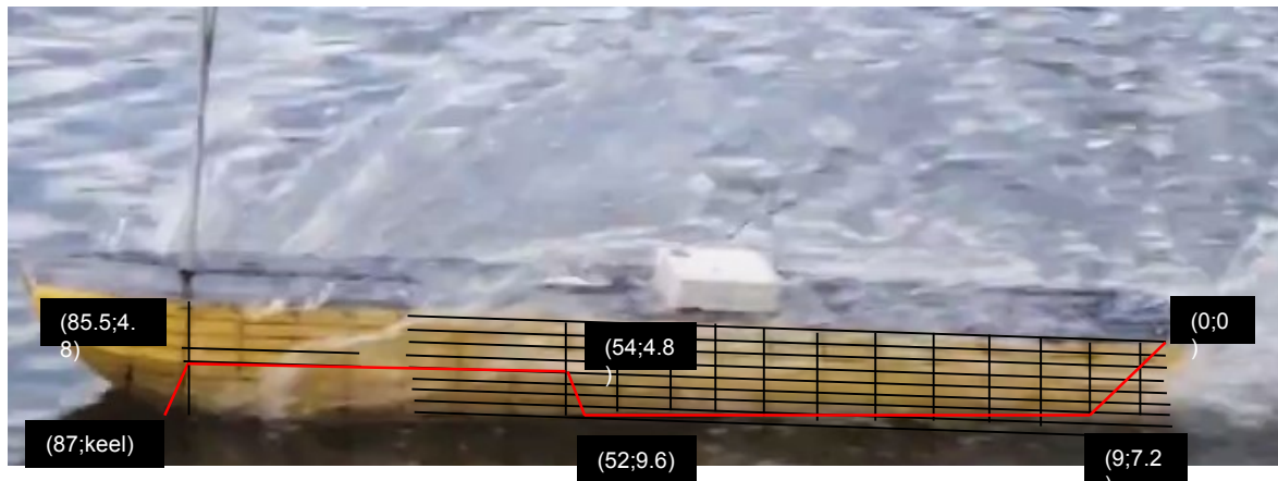
Figure E.19: Wetted area measurements (in centimeters) of the wetted area for the hysucat at a real scale speed of 20 m/s. Wetted area = 18.56 \text{ m}^2 . Wetted keel length = 6.96 \text{ m}
