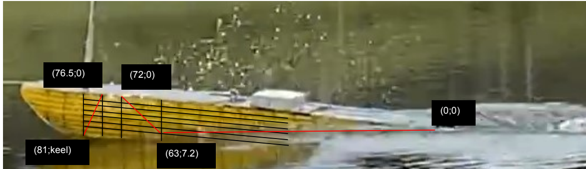
Figure E.15: Wetted area measurements (in centimeters) of the wetted area for the hysucat at a real scale speed of 10 m/s. Wetted area = 21.76 \text{ m}^2 . Wetted keel length = 6.48 \text{ m}
