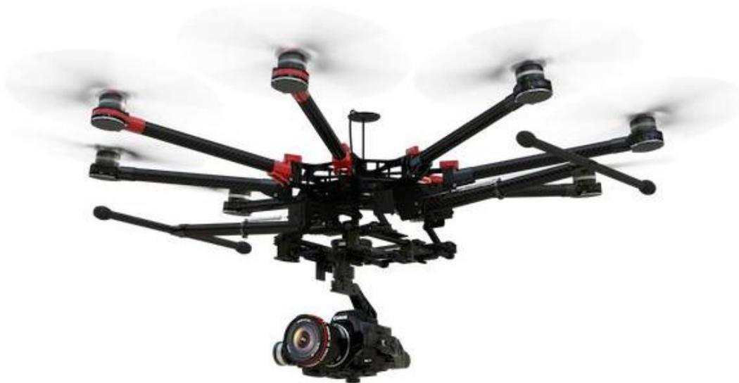
**Figura 5. Octorrotores DJI S1000 (DJI, 2015).**
