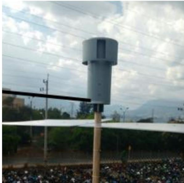
Figure 3.2: Sigma-2 particle sampler.
