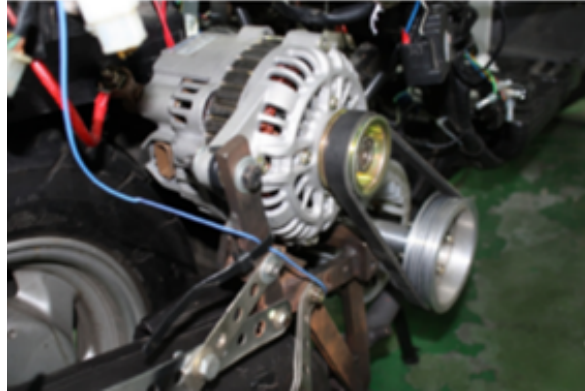
Figure 2.14: Generator included in the prototype by Wu et al. (2013)
