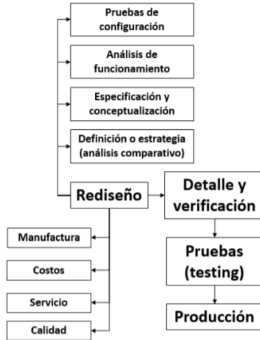
Figure 2.5: Sequential structure of production-oriented product redesign methodology by (Escoto and López Parra, 2019)
