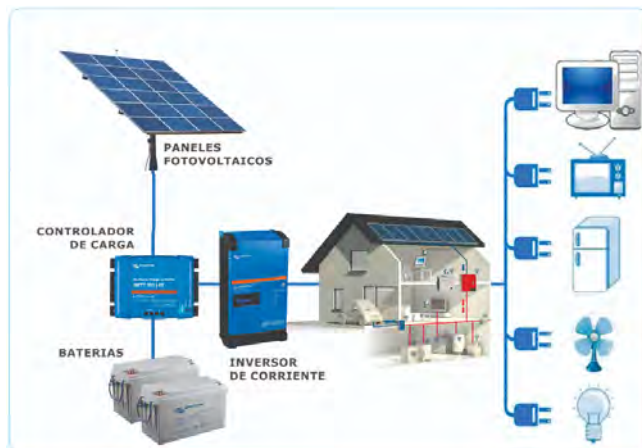
Figura 2.2: Sistema off-grid (Green Energy, 2023)
