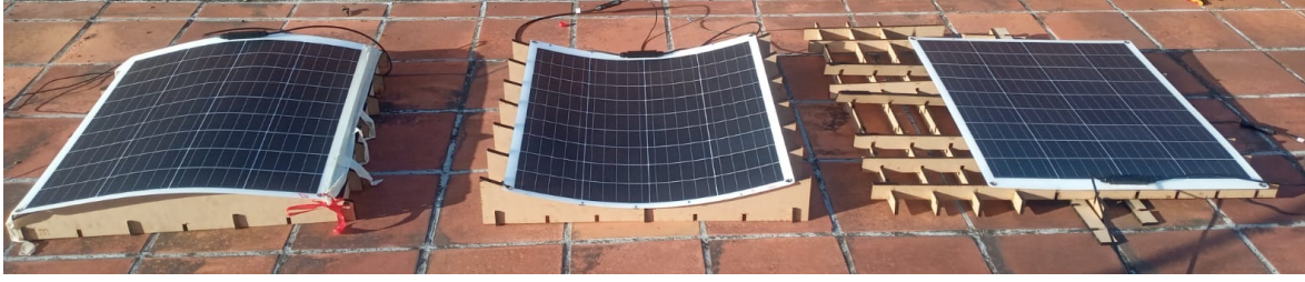
Figure B.6: Test of commercial PV modules with curved geometry
