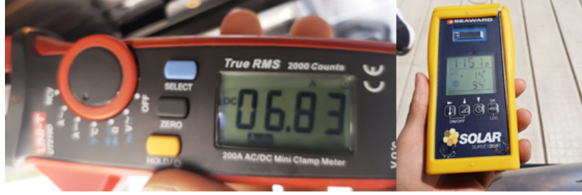
Figure 5.26: Irradiance and current measured in boat operating site
