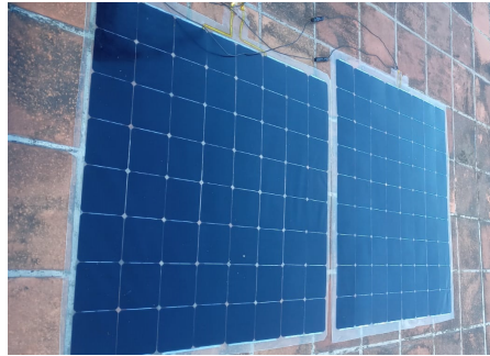
Figure 6.20: Test of fabricated PV modules with flat geometry
