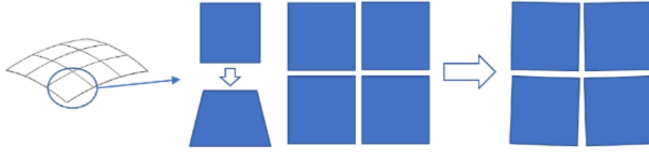
Figure 3.7: Deployment of a flat PV module on a curved surface (Ota et al., 2022b).
