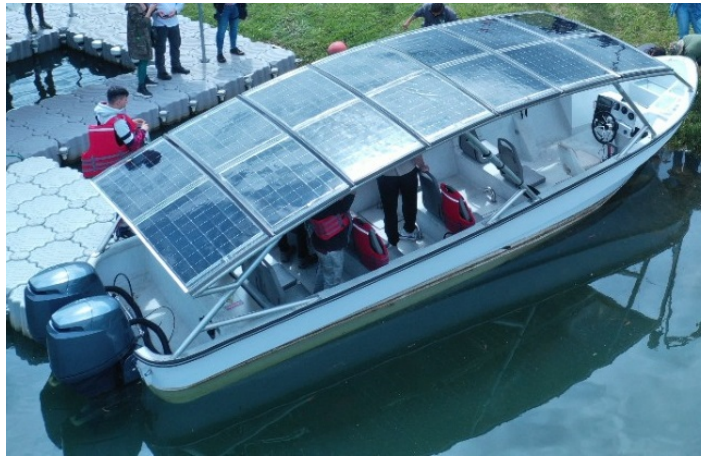
Figure 5.25: Materialization of PV array of electrosolar boat
