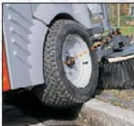
Can negotiate kerbs without difficulty thanks to the hydrostatic drive to the large front wheels.
