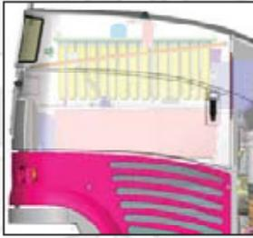
The newly developed dry filter system cleans the used air with a degree of separation of 99,5%. This guarantees that the machine can be used in public areas without dust emissions affecting passers-by.
