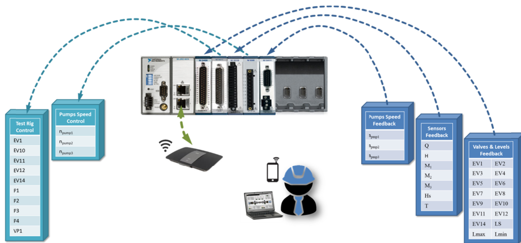
Fig. 5. NI cRIO-9074 [10] automatic controller and the managed test rig I/O variables.
