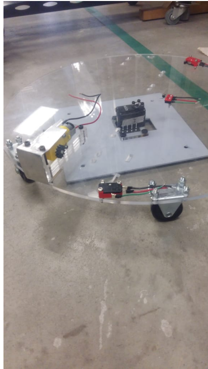
Fig. 10.14.: Motors, micro-switches and wheels on the rotary platform.
