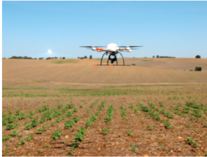
Fig. 5.12.: UAV equipped with RS devices for evaluation of weed infestation [45].
