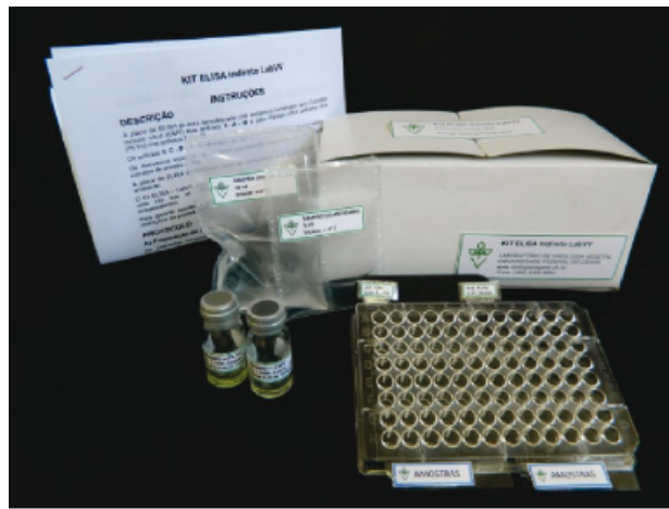
Fig. 5.8.: Simple ELISA kit developed at the Plant Virus Laboratory from Federal University of Ceará, Brazil [44].
