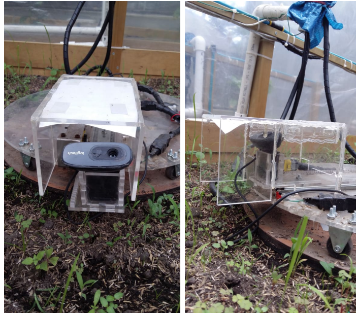
(a) Front view of the the web- cam assembly. (b) Side view of the the web- cam assembly.
