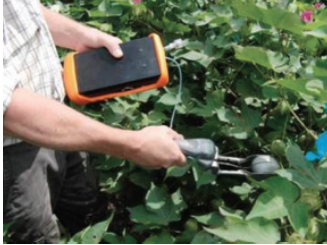
Fig. 5.11.: Field sampling cotton bolls with a pest and damage detector developed to draw VOCs [50].
