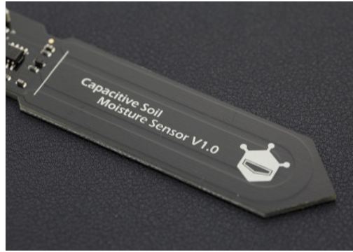
Fig. 9.13.: Analog capacitive soil moisture sensor [97].
