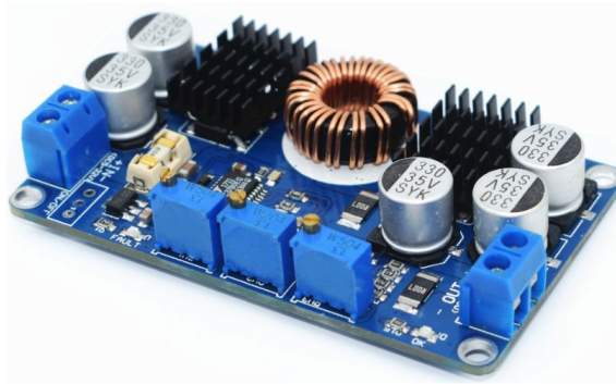
Fig. 9.21.: Buck-boost switching regulator [109].
