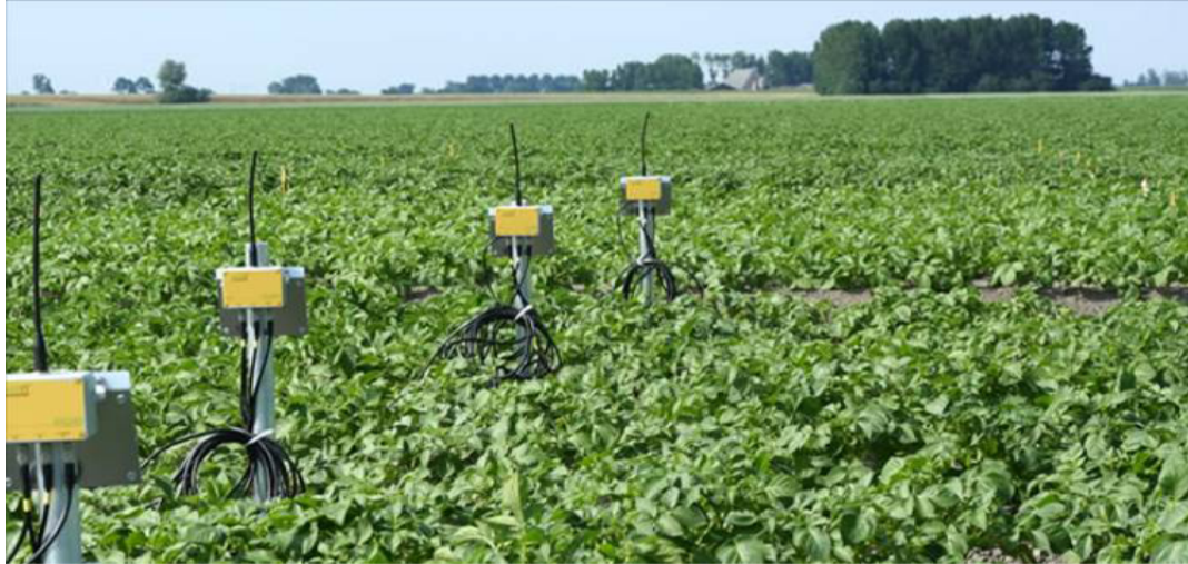
Fig. 5.14.: WSN in agriculture for water management [57].
