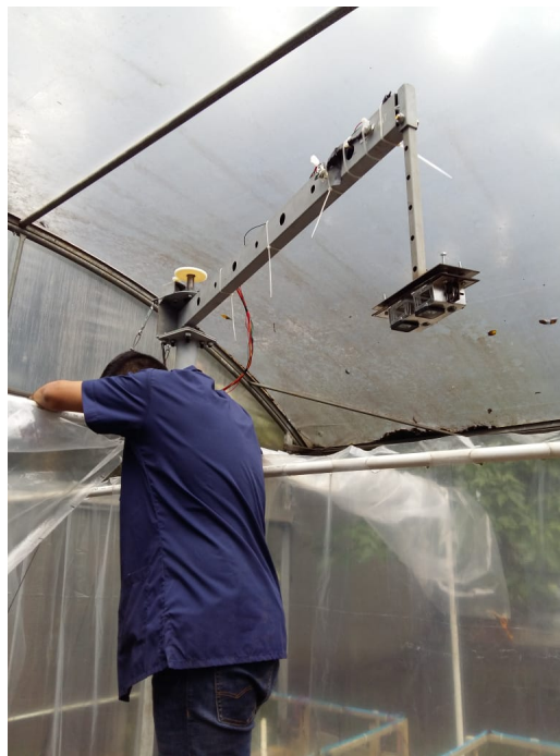
Fig. 10.7.: Installation of the multispectral cameras.
