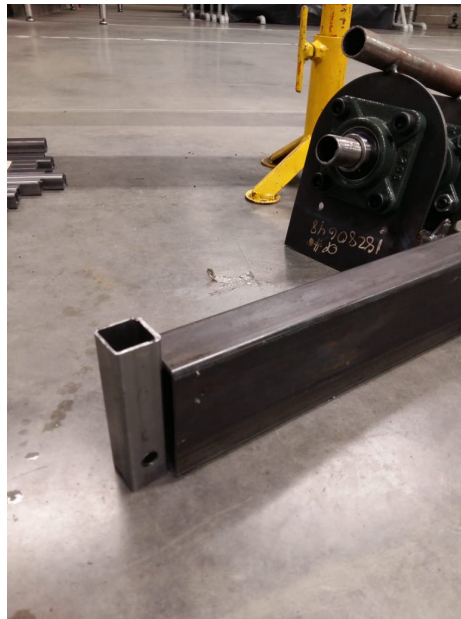
(b) Mounting point of the arm's profile for the multispectral cameras.
