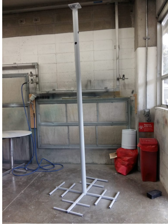
Fig. 10.3.: Finished rotary arm's support structure.
