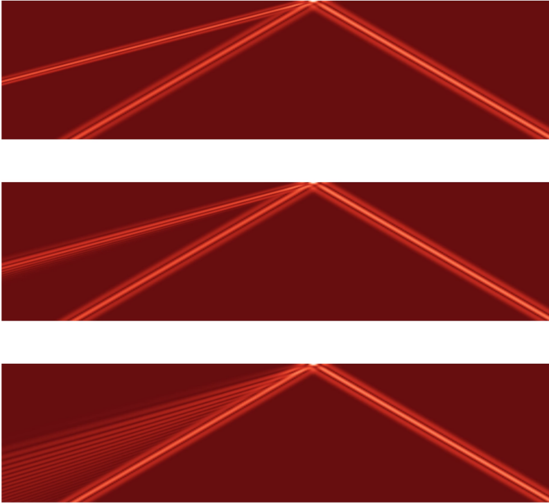
Figure 38: Reflection of an incident P-wave on a halfspace for different length scales. The angle of incidence is \pi/6 rad, the P-wave speed is c_1 = 2 , the (classical) S-wave speed is c_2 = 1 , and the length scales are l = \{0.01, 0.03, 0.1\} (from top to bottom). It is clearly seen how the dispersion increases while the length scale parameter increases.
