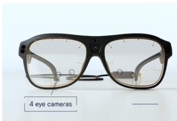
Figura 8. Gafas eye tracker Tobii Pro Glasses 3
