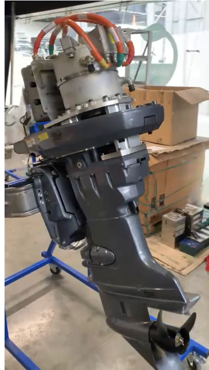
Figure 4.13: Outboard Electrical Unit: Physical Prototype Implementation
