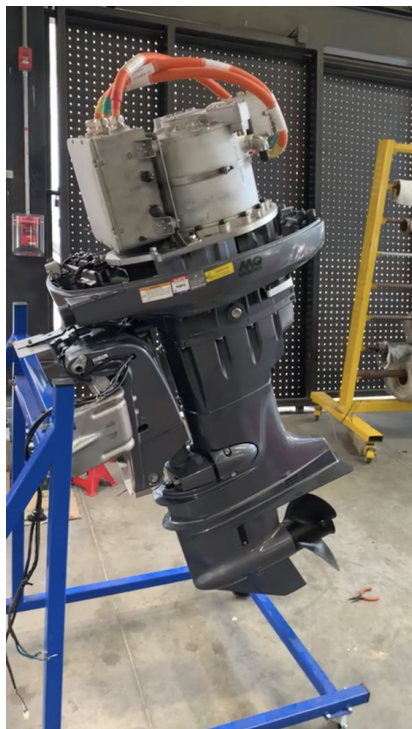
Figure 4.13: Outboard Electrical Unit: Physical Prototype Implementation
