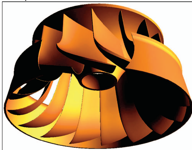
Figure 1: CFD-Based optimization result of a turbine runner.
