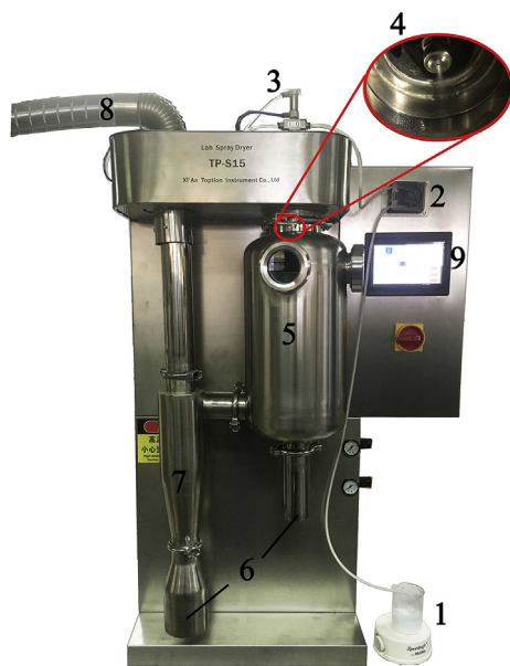
Fig. 2. Image of Toption TP S-15™ spray dryer. 1. Slurry, 2. Peristaltic pump, 3. Slurry inlet to the nozzle, 4. Nozzle detail, 5. Drying chamber, 6. Collector cup, 7. Classifier cyclone, 8. Exhaust pipe, 9. Control panel
