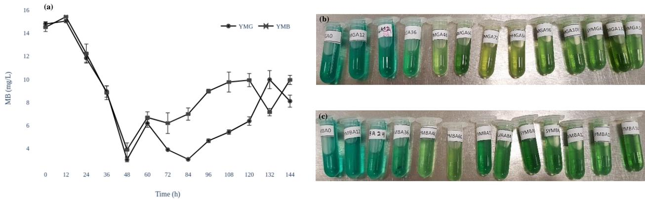
Figure 7. (a) Variation in MB concentration over time. (b) Samples of the kinetics of YMG medium with MB, without added yeast. (c) Samples of the kinetics of YMB medium with MB, without added yeast.
