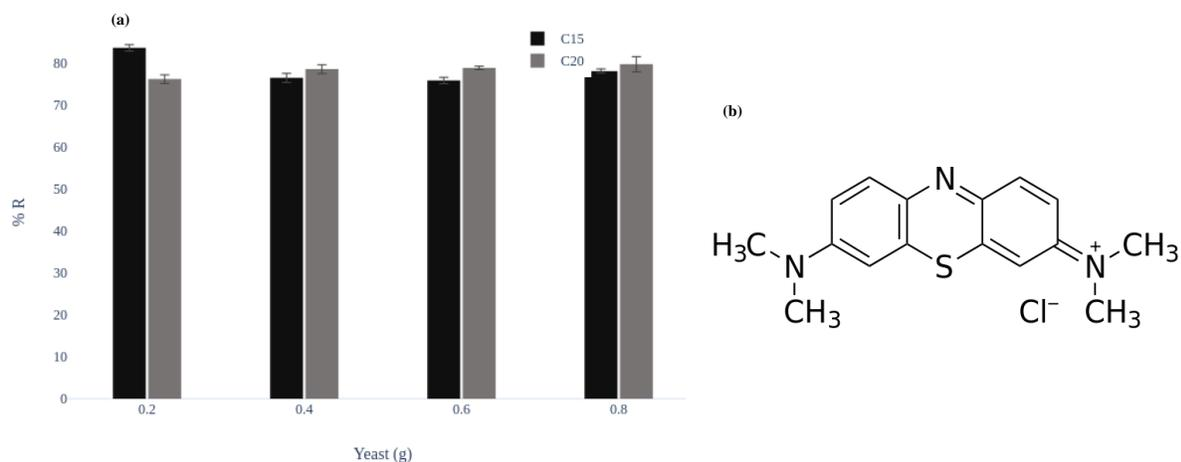
Figure 3. (a) Effect of concentrations of dried cultivated biomass on its capacity of MB biosorption. (b) Chemical structure of MB.
