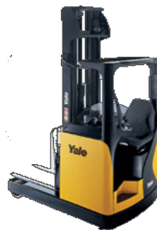
Figura 2. Montacargas de doble alcance, Yale:MR14/ MR14H/ MR16.
