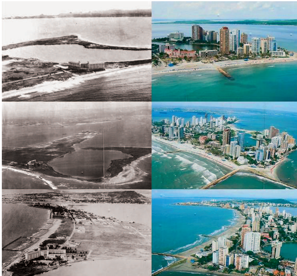
Fig. 2. Aerial view of coastal occupation and groin fields (“domino effect”) at Bocagrande, El Laguito and Castillogrande sectors (Cartagena City). The images on the left side correspond to 1950s, the ones on the right correspond to 2005 (courtesy of Historic Archive of Cartagena de Indias)
